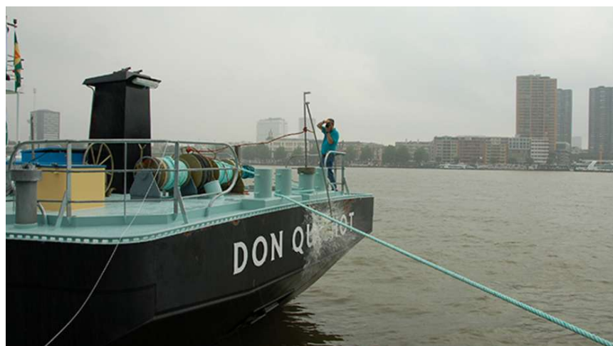
First floating degassing station for inland waterway vessels: MTS Don Quichot (GreenPoint Maritime Services) Source: Port of Rotterdam Mathijs Schoon
